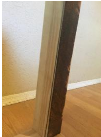
Figure 27: Burn Marks from Circular Saw
