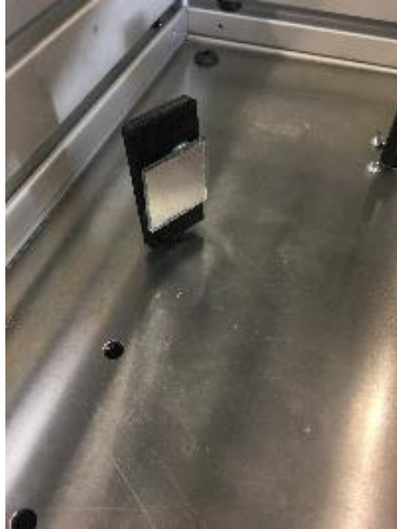
Figure 23: Drilled Holes for Mirror Post
