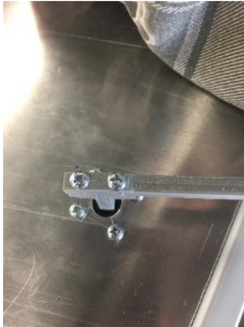
Figure 19: Drilled and Tape Holes on Hand Crank
